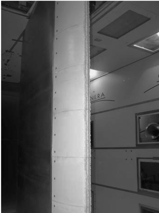
Fig. 8 Completed installation of horn shape EG1164 casting sections on the leading edge of the NACA 23012 airfoil model (upper-surface view).
